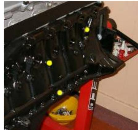
Use the RB20/25/26's oil dip stick & holder as the RB30's is not long enough to clear the DOHC inlet manifold.
