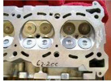
As a reference point the RB30's SOHC head cc's up around the 55 to 58cc mark.
