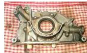
Ensure you use **lock tight** on the bolts when assembling the oil pump as they are known to rattle loose causing a gradual loss of oil pressure.
